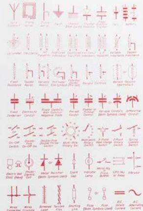
Conventional signs used to draw a wireless circuit, which rarely coincide of a number of their signs placed together. Picture taken from 'A Beginner's Guide to Radio' by F. J. Collins.
